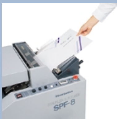
Insert prints, align the side guide, then press the start button.
